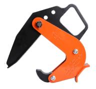
The Tiger CPL pipe lifting clamps are used in sets of three for the vertical transportation of concrete pipe sections with a diameter of up to 2m. The jaw capacity is designed for pipe thickness of 40-120mm for the 1.5t capacity set and 90-220mm for the 3.0t capacity set. Attachment and removal of the clamps from the pipe is extremely easy due to the simple and straightforward design. For concrete according to DIN4034. The capacities shown are based on a set of three clamps.
